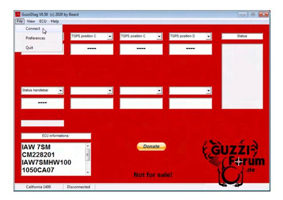
You will be asked to switch the ignition key switch to 'on'. Do not start the engine.
