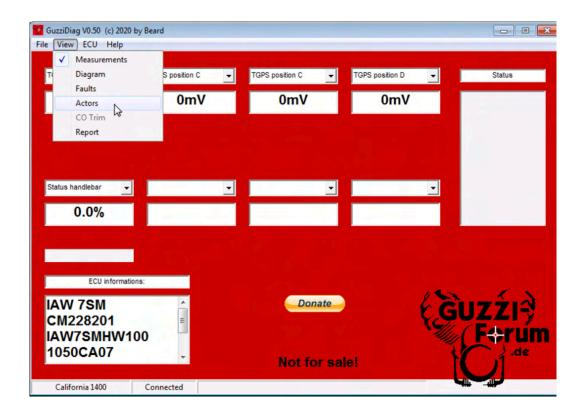
To reset the Autolearning Parameters, scroll down and select 'Reset autolearning parameters'.
