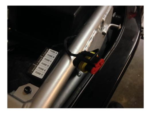
Attach the clips from the 3 pin cable to the battery (take note of polarity) and plug the USB cable into a USB port on your computer.
