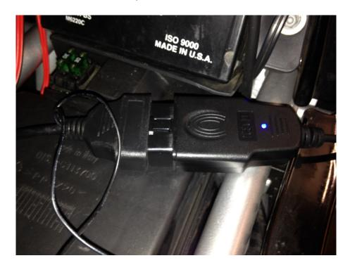
To read and backup your existing map, open the Reader. Your computer may have multiple COM ports, so select the correct one from the drop-down box. it is usually the last one or highest number. if it doesn't connect at first, keep trying different ports. In my example, I only have one, COM4.
